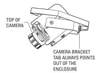
**Ceiling Mounting** — The camera bracket tab points out of the enclosure and the top of the camera is pointed in the opposite direction.
